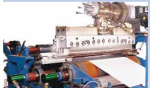
*Orange overcoat masking tape on chill roll*
