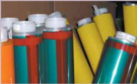
*Pressure sensitive tape logs secured against unwind*
