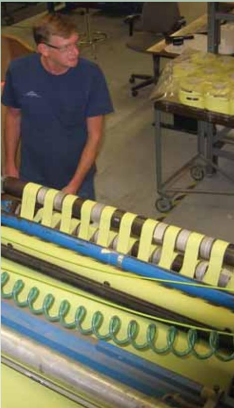
*Tape conversion operator on crush-cut, rewind slitter*
